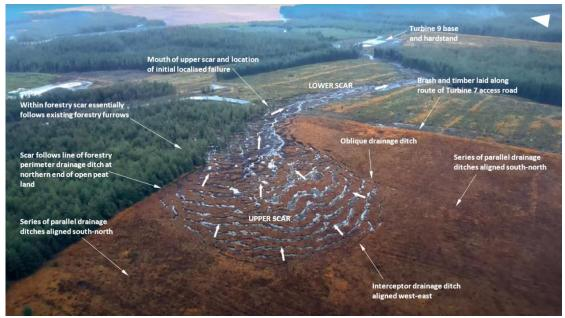
Figure 7.1 Peat failure location
